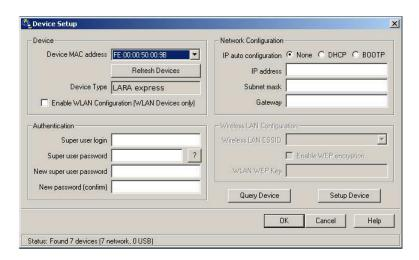
On the upper left corner, the MAC address of the LARA express is displayed. To detect the MAC address manually, press the button "Refresh Devices". The displayed MAC address is the same MAC address printed on the white sticker placed on the back of the LARA express. If the LARA express is connected via USB, it is classified as an USB device and an appropriate drive letter is chosen for this device.
